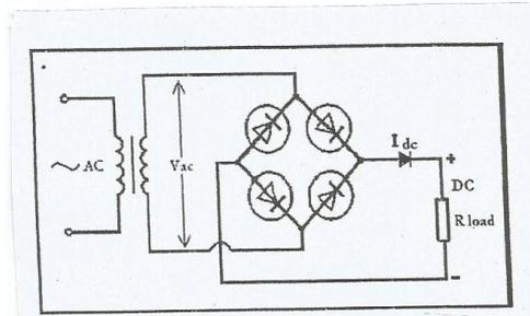
**Figure 2: The Bridge rectified circuit**
